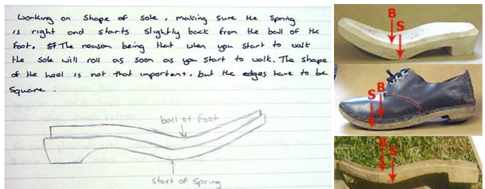
Figure 66 Above: clog sole drawing from Parfitt's notebook. Right: soles made by (from top) Atkinson, Edwards and James showing start of spring (S) and ball of foot (B).
